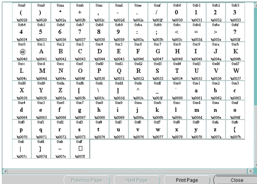
Figure 13–18 US7ASCII Code Chart
